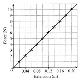
This graph shows the relationship between the extension, in m, of a spring and the force, in N.
